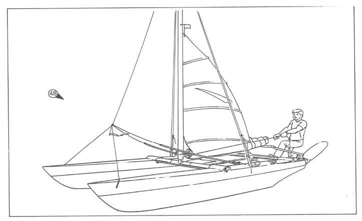
\* Check that the halyard is running up the line of the mast groove, NOT AROUND THE MAST HOOK, and raise the sail by pulling the halyard where it exits from the base of the mast (Fig 48). The mainsail is secured at the top of the mast by the halyard lock and the last 15cm of mainsail hoist should be achieved with a firm pull to ensure the locking ring is positioned over the hook as shown (Fig 49).
